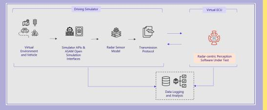
The Aptiv virtual simulation framework for testing radar-centric perception stack is composed of a virtual Driving Simulator and a Virtual ECU, which executes the software components.
