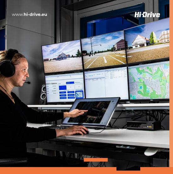
A teleoperator using the prototypical workplace for teleoperating CAVs at DLR's Institute of **Transportation Systems**
