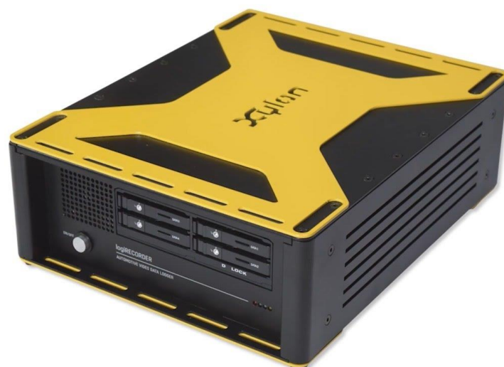
Figure A2.27: Xylon logiRECORDER Video Data Logger for Automotive Applications [27]
