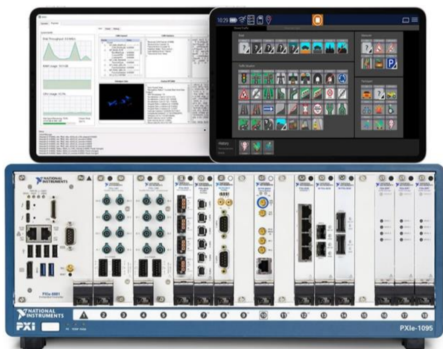
Figure A2.17: NI Data Record System AD - Hardware and Software GUI [19]
