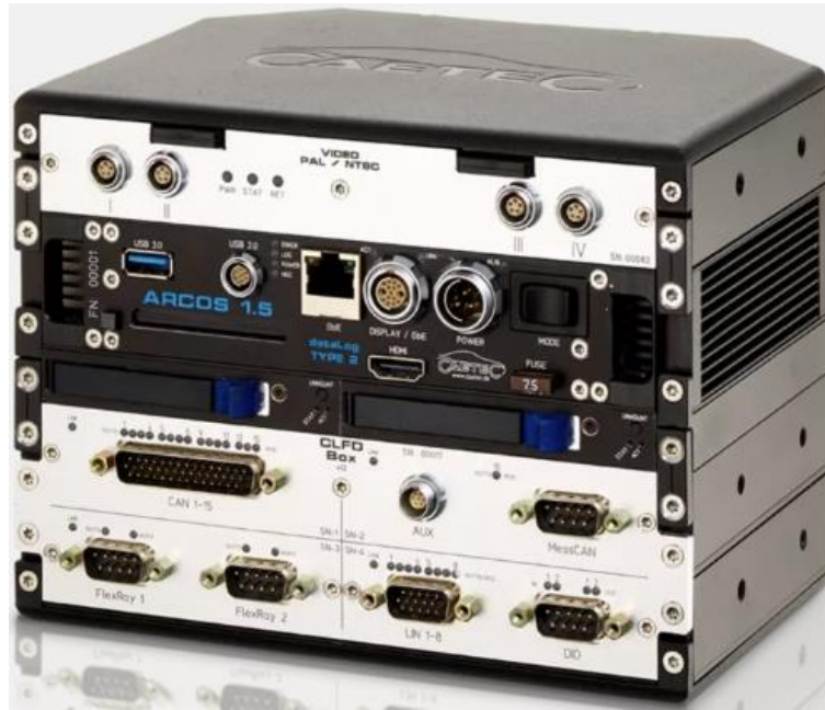
Figure A2.13: ARCOS 1.5 high scalable data logger for automotive networks [15]
