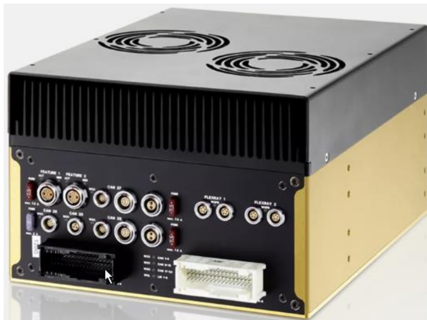
Figure A2.14: ETHOS high performance data logger for ADAS/AD applications [16]
