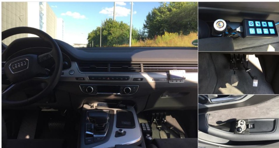
Figure 4.22: Modified WOZ vehicle for WIVW / Audi test-track study (Method ID: TT03)
