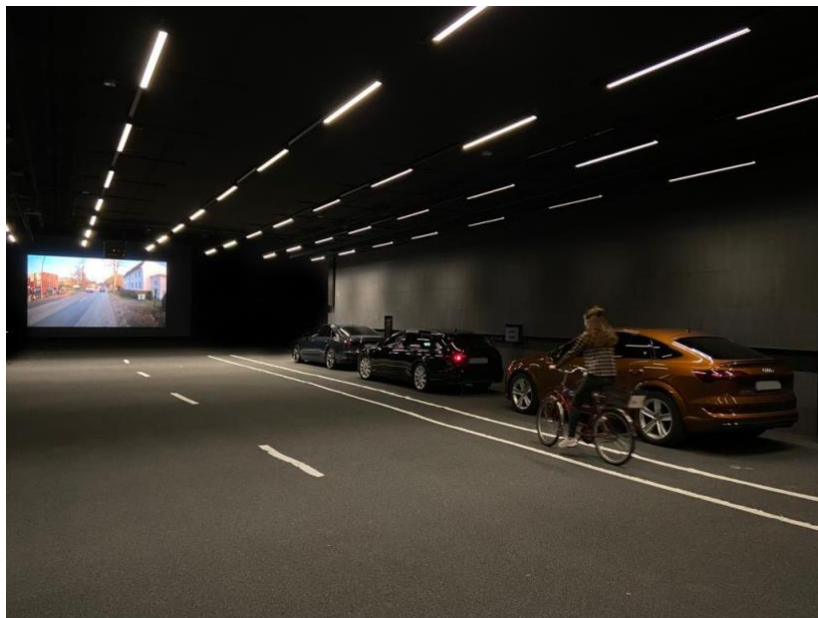
Figure 4.23: Audi test setup for the evaluation of hazard warnings (Barthleme, 2023; Method ID: TT04)
