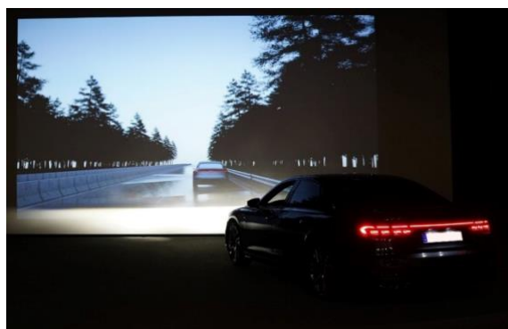
Figure 4.13: Hybrid setup for the evaluation of hazard warnings in the Audi driving simulator (Kraft 2022; Method ID: DS08)
