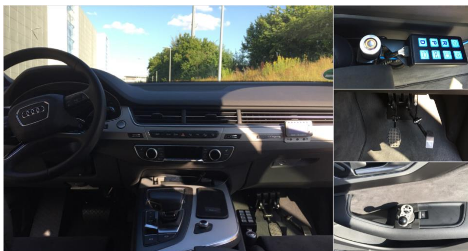
Figure 4.22: Modified WOZ vehicle for WIVW / Audi test-track study (Method ID: TT03)
