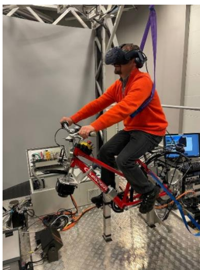
Figure 4.18: A participant riding the bicycle simulator at VTI, Sweden (Method ID: BS01)
