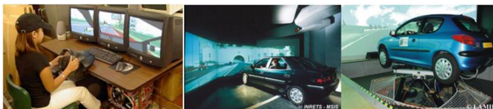
Figure 4.6: Examples of driving simulators( low-fidelity, image taken from Park et al., 2005, medium-, and high-fidelity, images taken from Auberlet et al., 2010)
