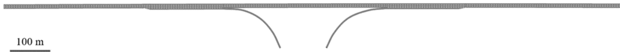
Figure 3.10: Schematic example of a motorway section for traffic simulation. The section extends beyond the figure for about 1.5 km in both directions.
