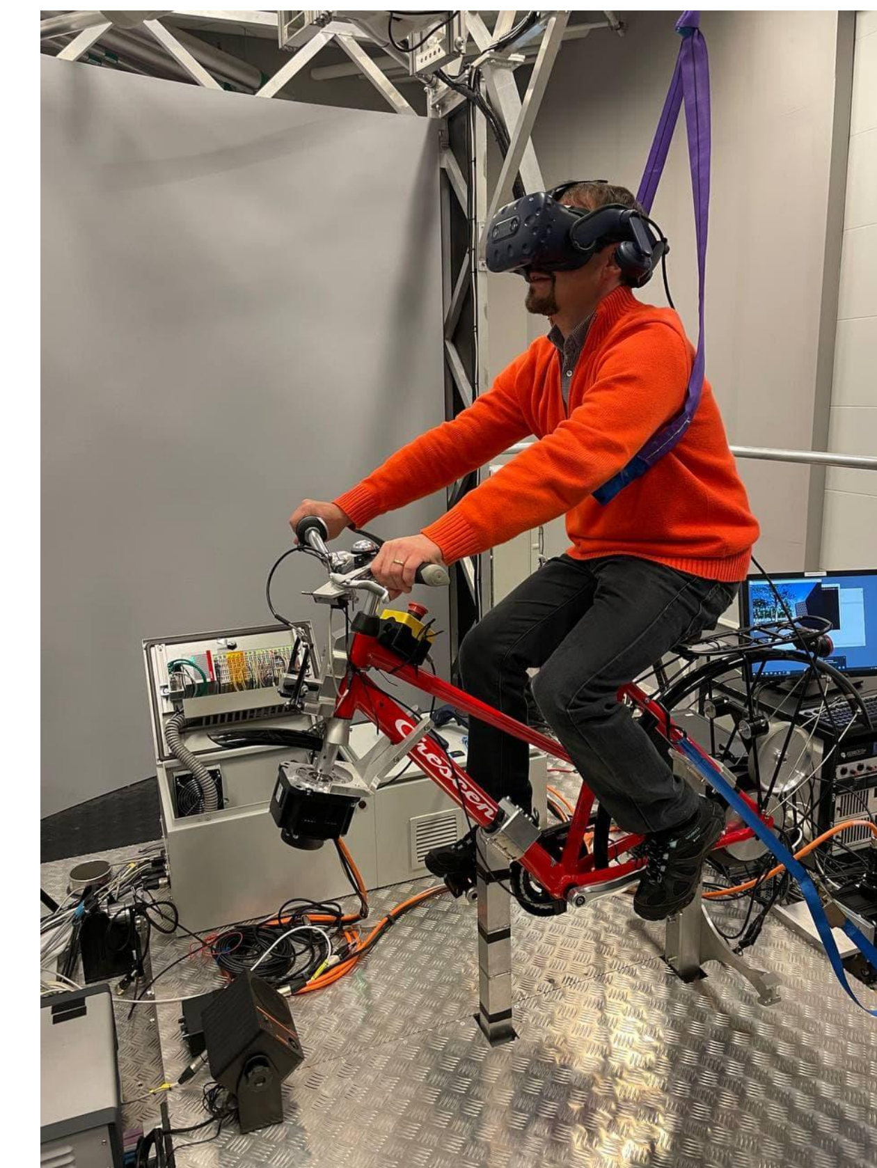
Fig. 3: Bike simulator compartment at VTI facilities
