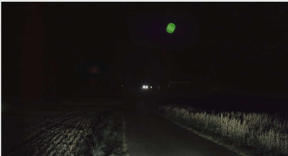
High End Color-Camera with low beam headlights : Only the first 50m are visible OnSemi Aptina AR0230, resolution: 1920x1024
