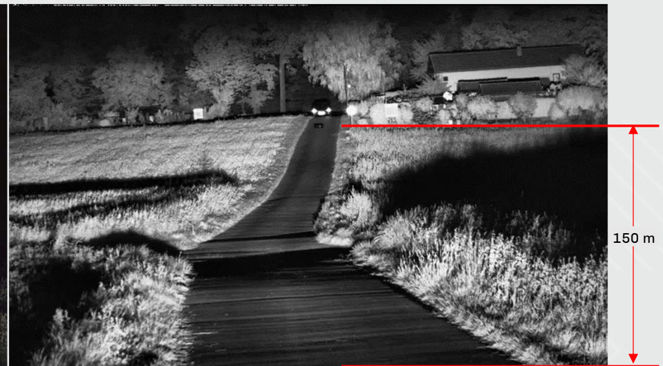
Gated Camera from BWV: The tire at 155m distance can be seen well! Resolution – 800x480
