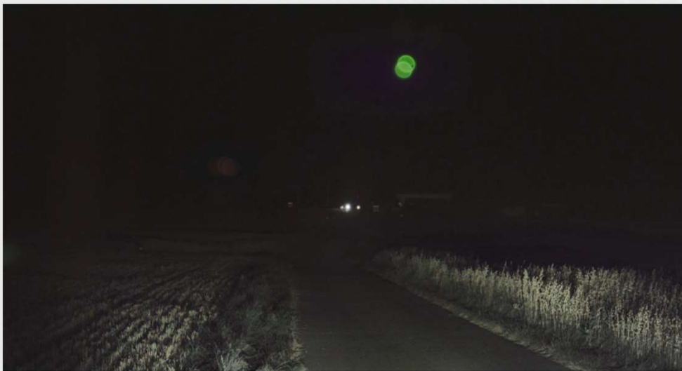
High End Color-Camera with low beam headlights: Only the first 50m are visible
